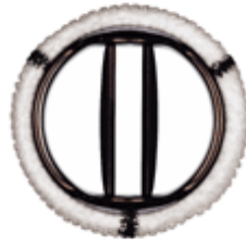
Figure 2.1 Bi-leaflet mechanical heart valve used for the tests.
