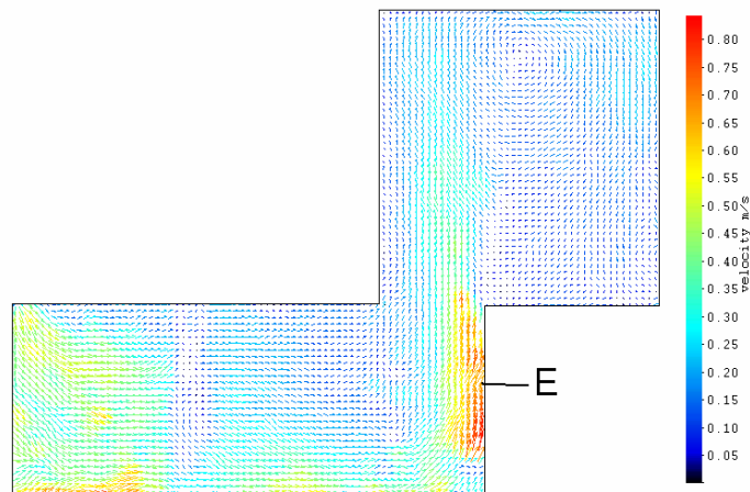
Fig. 13 Velocity vectors on a 90° plane (12 mm spool opening, 0.91 l/s flow rate)
