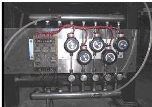
Fig. 3: Valve array for the air jets modulation.
