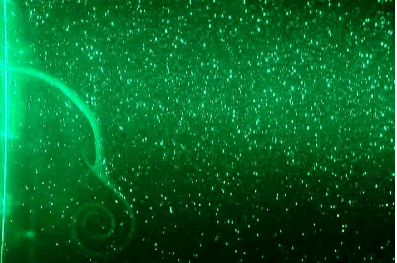
Fig. 8: Longitudinal flow visualization of the planar jet mixed with lycopodium at R=3 , Re_j=30 , U_\infty=1 cm/s ( f=0.33 Hz, St=0.011 ).
